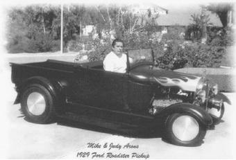
All steel body on a model A frame.; Painted flat black-and black tuck and roll by Joel's Interior Rear fender by Ralph (the old blister) Knight. 4 inch dropped front axle with disc brakes, and 8 inch Ford rear axle with coil over springs. 1947 Ford
