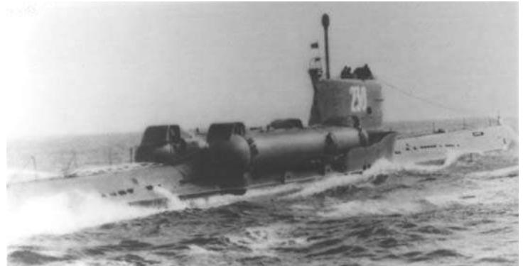
Later Whiskey class variants known as "Long Bin" modifications involved elongation of the sail with the capability of carrying four missiles stored at an angle permitting direct launch from the tubes. Unlike the Regulus submarines, the Russian launch system did not require handling of the missiles on deck prior to launch. Six of the "Long Bin" variants were built.
