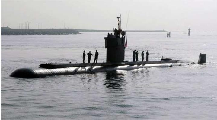
*Dolphin* was a unique, special purpose submarine not designed to be a weapons system, but as a deep diving test platform. With a test depth in excess of 3,000 feet, she was able to test systems and equipment at depths well beyond that at which other submarines could operate. The pressure hull was a round cylinder with hemispherical end caps and a minimum of hull penetrations.
