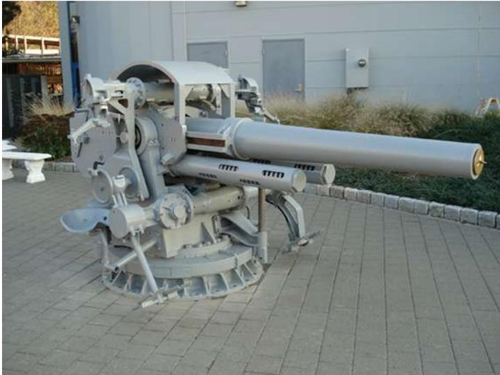
The 5"/25 deck gun constructed largely of corrosion resistant metal was designed especially for use on submarines. Its 125" gun barrel was short by comparison to other naval 5" guns, but longer gun barrels would be advantageous only for more stable platforms and the shorter barrel was well suited for submarine use. It was capable of firing a 54 pound projectile 18,000 yards.
